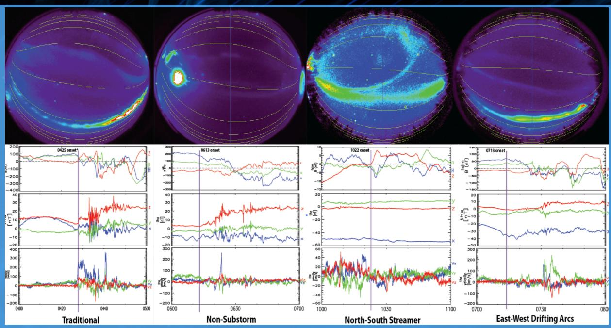
Plots are (top to bottom): white light ASI, ground magnetometer readings, THEMIS magnetic field strength, and THEMIS bulk plasma velocity readings for example events of 4 main subcategories. Each type has distinct characteristics, suggesting different causes for the visual phenomena pictured.
